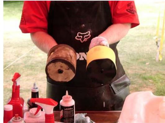
Water and spray cleaner pre rinsing a filter extends the life of the filter washing solution. This also makes cleaning the filters easier and faster. Always clear rinse the filter thoroughly after cleaning. This removes the cleaner and any grit that that is trapped in the cells.
