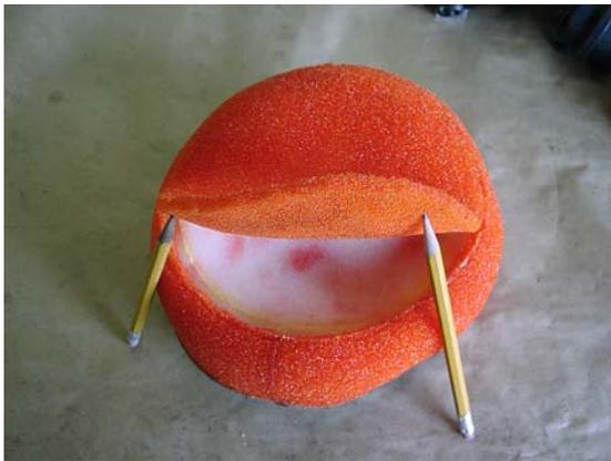
Air filter de lamination can be caused by strong cleaners and solvents attacking the glued seams. Always check the filter for damage. Foam filters do wear out!
