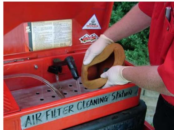
When you have cleaned the filter in solvent use paper towels to blot dry the foam. Then wash the solvent residues from the foam element with warm water and a good detergent such as Hondabrite®, Simple Green, dish soap or other household cleaner. Be sure to rinse all of the soap suds out of the element.
