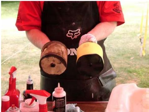
Cleaning the air filter element in water is easier on the foam and the filter will last longer. (Tip: If you run out of the special Honda air filter cleaner do not use solvent, try various laundry detergents and hot water.)
