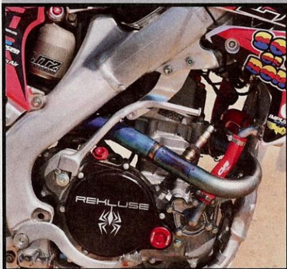
Motor-wise, the moto machine was strong, a Rekluse standard basket was used and larger ICW radiators were fitted.
