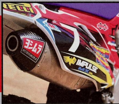
Yoshimura pipes were fit to both the MX and GNCC machine. Power gains from mid-to-top peak and a lighter weight were noticed.
