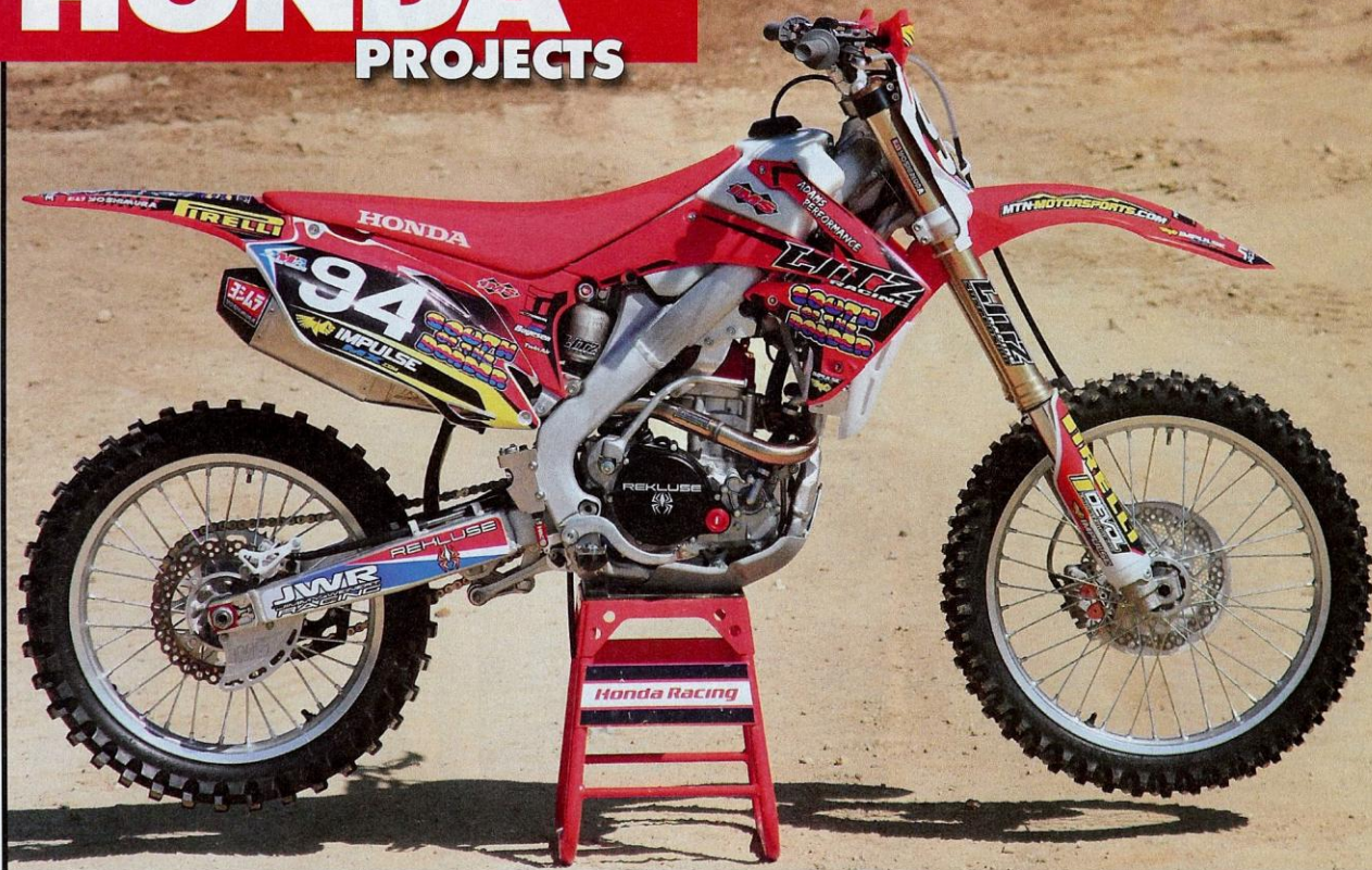
The major differences between the moto wagon and GNCC bikes came in suspension, the larger IMS tank and clutch. The GNCC bike used stock wheels and a stainless steel Yosh exhaust.
